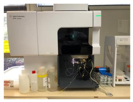
The ICP has stringent quality control systems built into the software, allowing for consistency and repeatability with all analyses. The simultaneous analysis of elements (up to 33 elements at one time) greatly reduces analytical time, allowing for fast turn-around of results.
